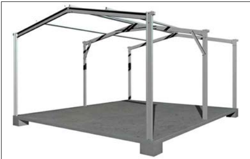
2B COMPLETE PORTAL FRAME ASSEMBLY 1 REFER 2C FOR TEMPORARY BRACING LOCATION
